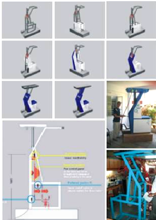
CNG dispenser with strong internal structure that forms a core functional chassis
